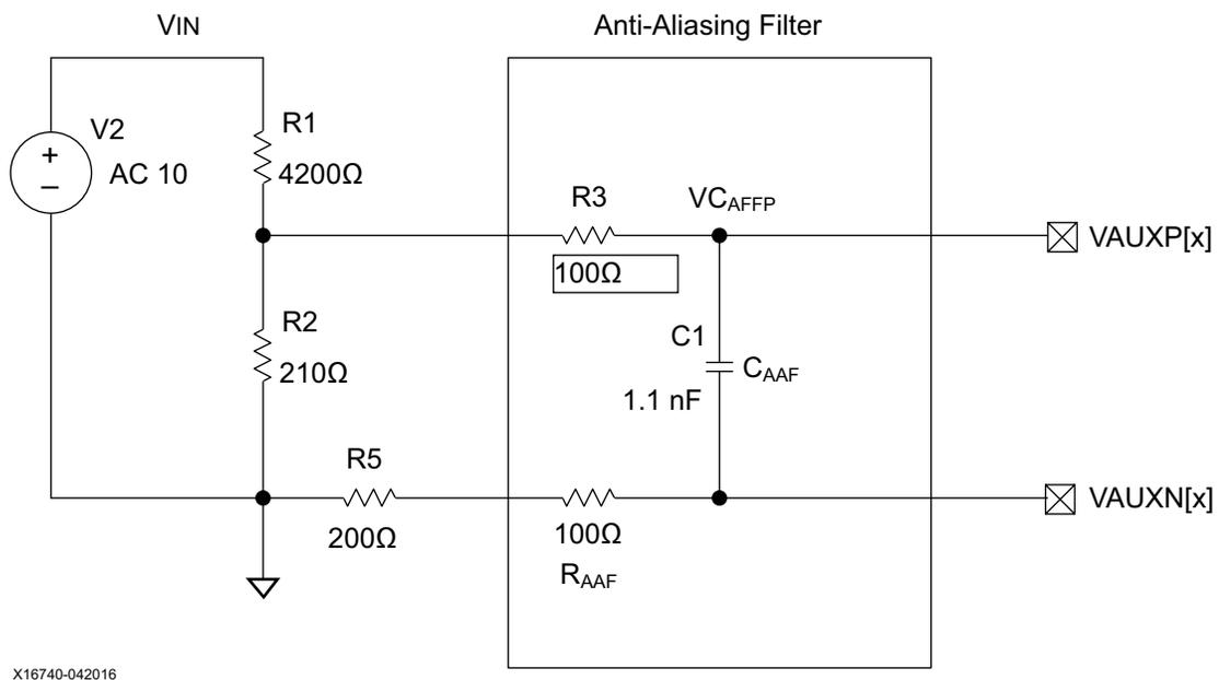
Figure 5-3: Voltage Attenuation
