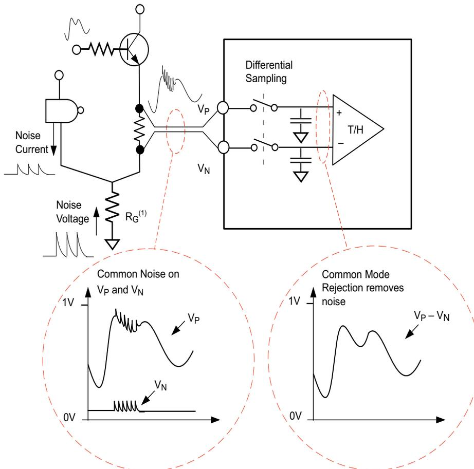
Note 1:  $R_G$  is common ground impedance.
