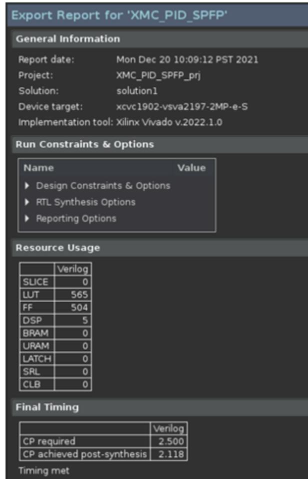
Figure 8: HLS Toolbox PID Single Precision Floating Point HLS Implementation Results
