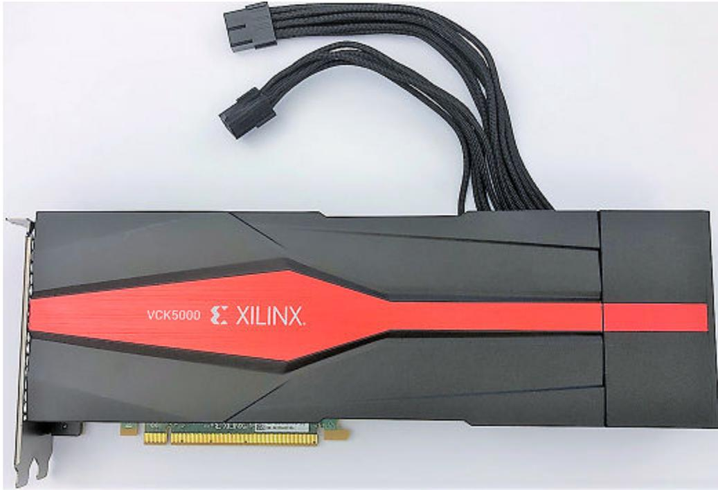
When the fan assembly is removed, it is referred to as the passive configuration. The passive cooling configuration requires external air flow to provide direct cooling to the card. Operation of a passively configured card without external cooling will cause damage to the card.
