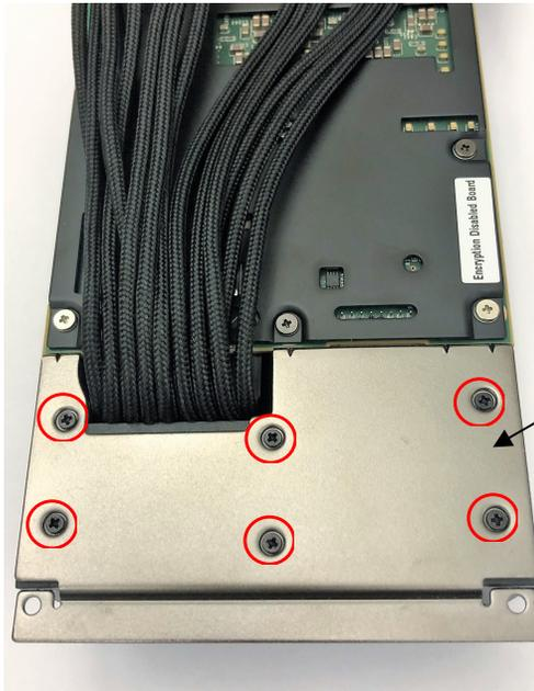
Metal Fan Assembly Mounting Bracket
