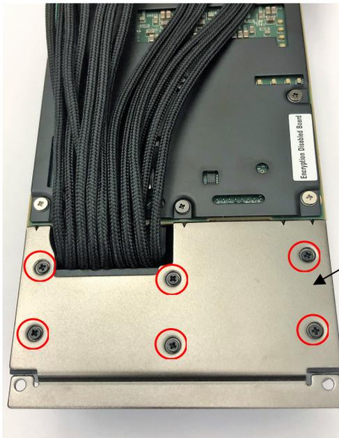
Metal Fan Assembly Mounting Bracket
