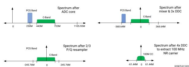
Figure 11: Baseband Spectrum at Each Stage of the DFE
