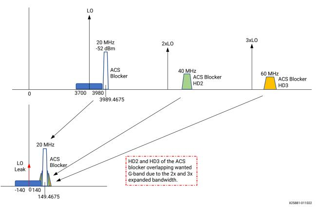
Figure 16: Adjacent Channel Selectivity Blocker with MxN Mixing Products
