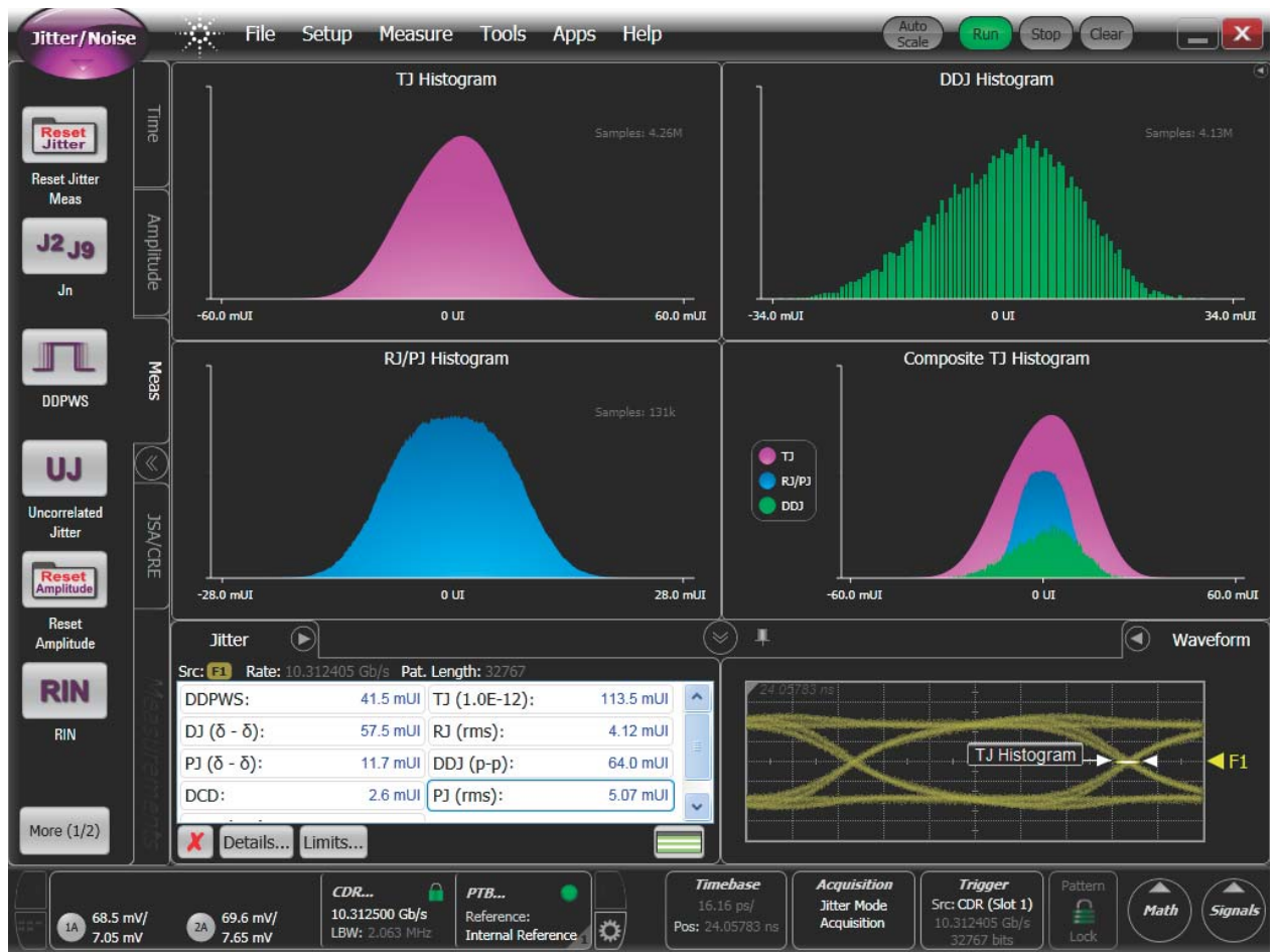
Figure 11: 10.3125 Gb/s Output Jitter Decomposition
