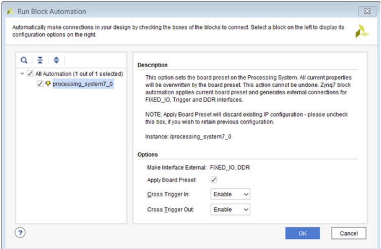
This enables the `TRIGGER_IN_0` and `TRIGGER_OUT_0` interfaces in the ZYNQ7 Processing System as show in the following figure.
