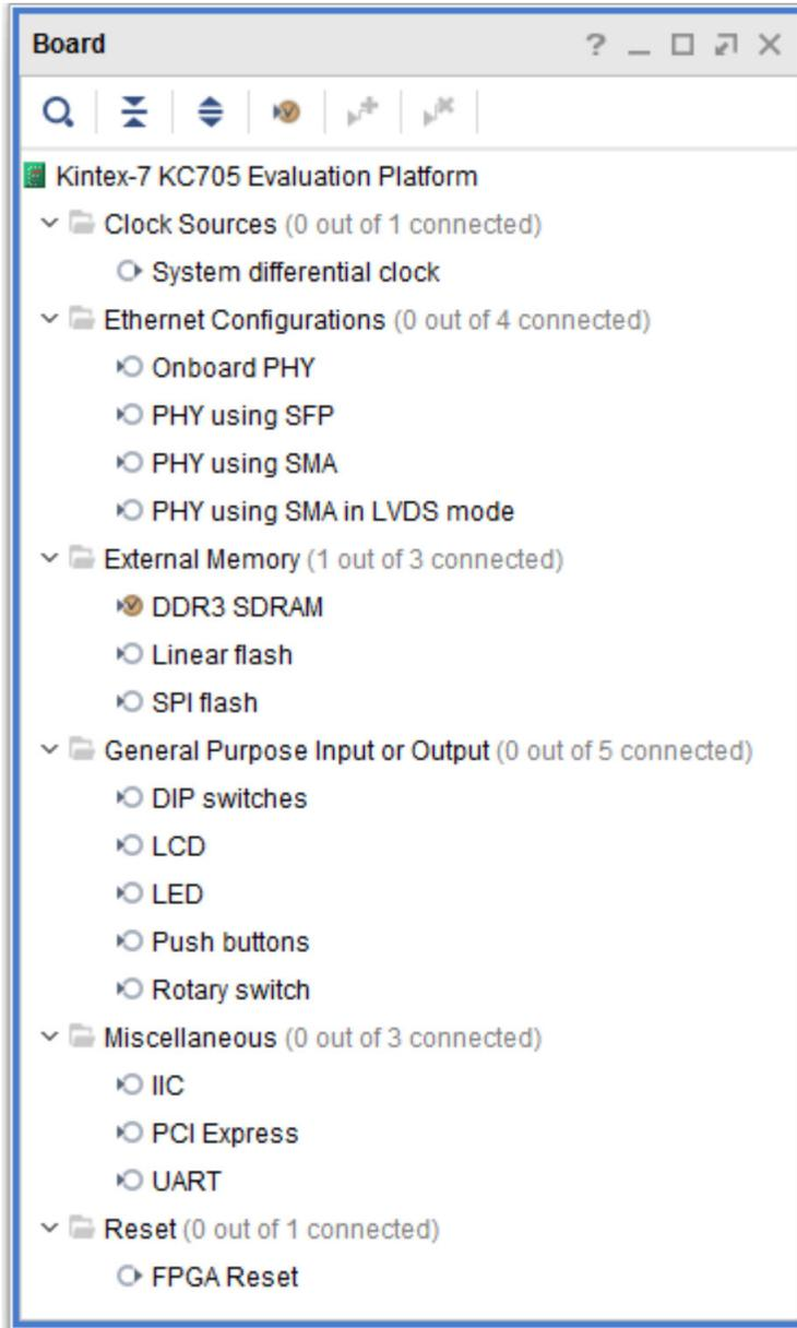
In the Board window, notice that the DDR3 SDRAM interface is connected as shown by the circle
