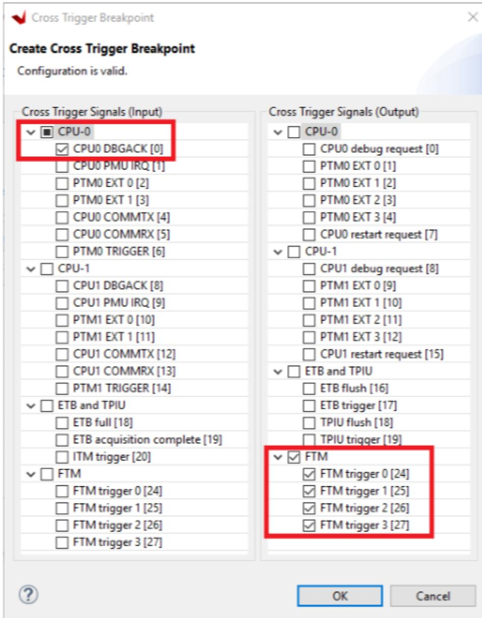
17. Click **OK**. This sets up the cross trigger condition for Processor to Fabric.
