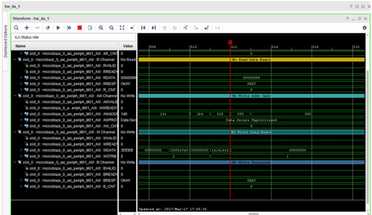
This demonstrates that when the breakpoint is encountered during code execution, the MicroBlaze triggers the ILA that is set up to trigger. This way you can monitor the state of the hardware at a certain point of code execution.
