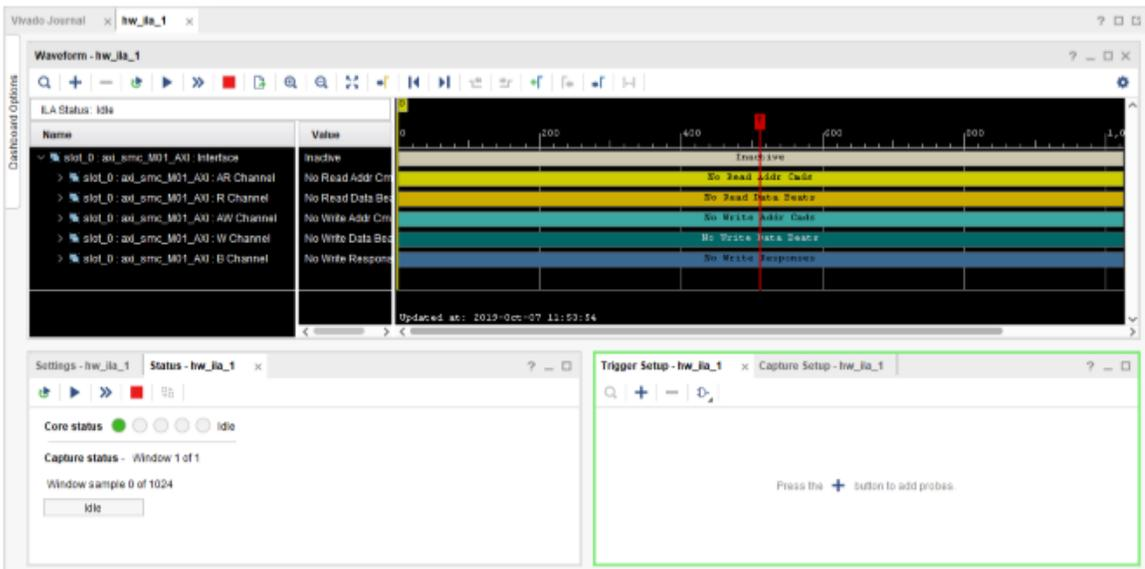
Expand some of the Signal Groups by clicking the drop-down to see Static data from the System ILA core in the waveform window as shown in the following figure.
