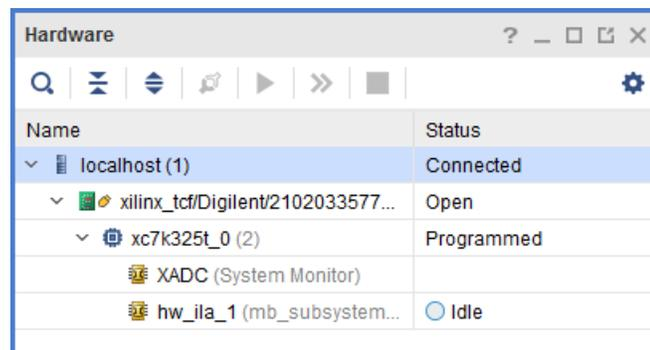
1. Select the settings - **hw\_ila\_1** tab and set the Trigger Mode Settings as follows:
