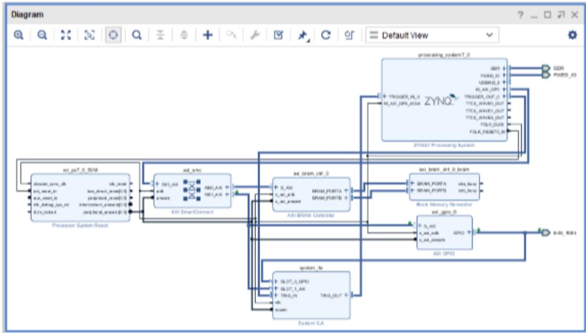
9. Click the **Validate Design** button to run Design Rule Checks on the design.
