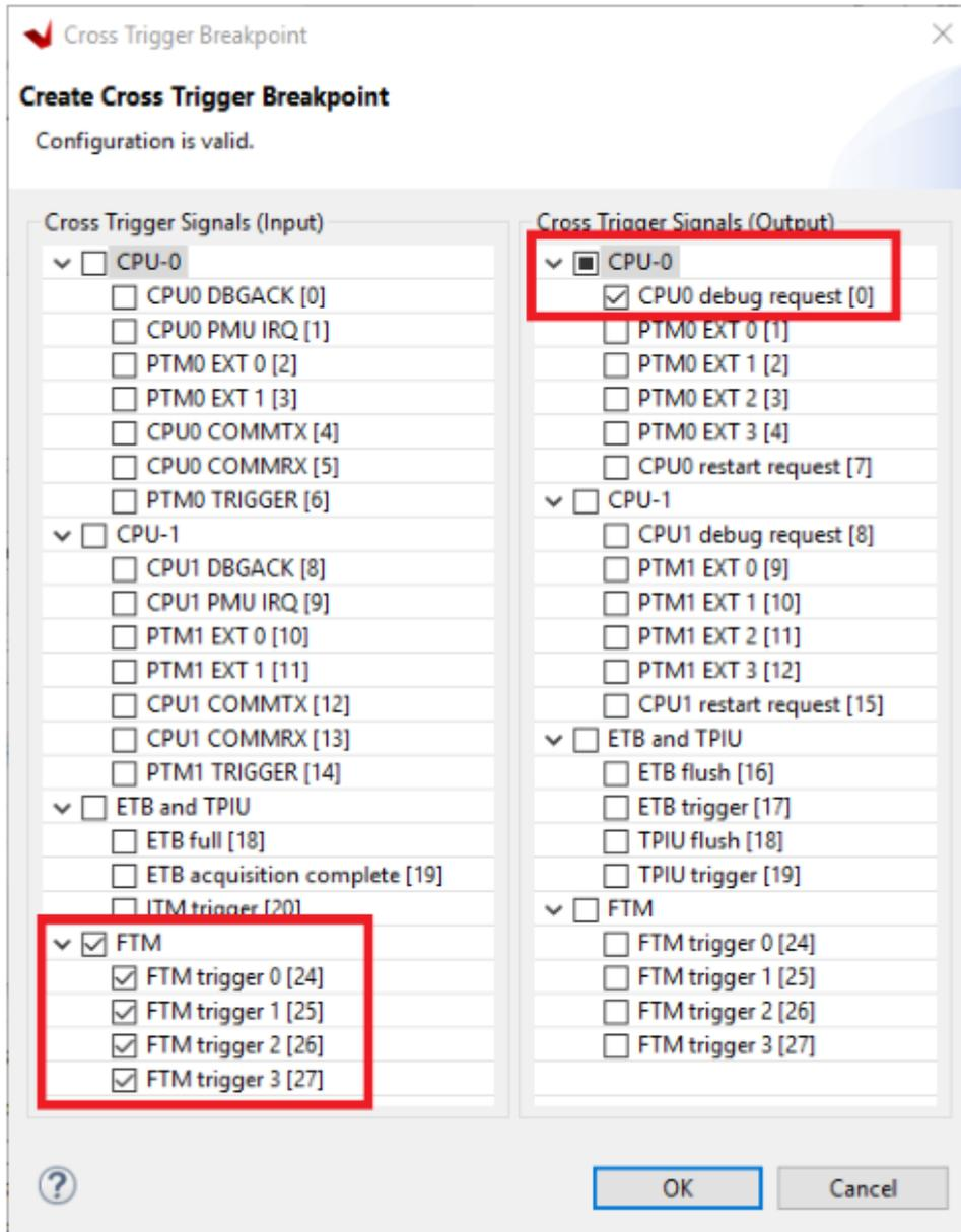
20. Click **OK**. This sets up the cross trigger condition for Fabric to Processor.
