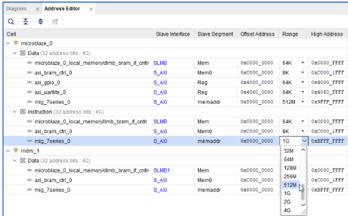
You must also ensure that the memory in which you are going to run and store your software is within the cacheable address range. This occurs when you enable Instruction Cache and Data Cache, while running the Block Automation for the MicroBlaze processor.
