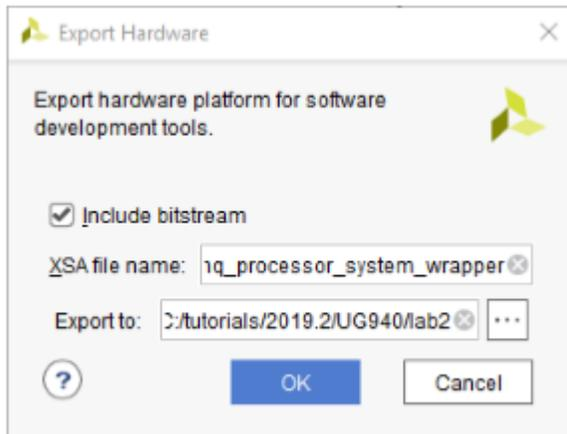
2. Ensure that the **Include Bitstream** check box is checked and that the **Export to field** is set to the default option.
