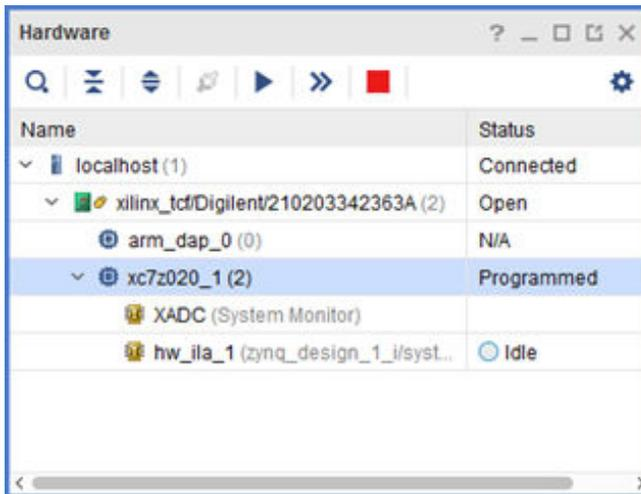
7. First, ensure that the ILA core is active and capturing data. To do this, select the Status tab of the `hw_ila_1` in the Hardware Manager.
