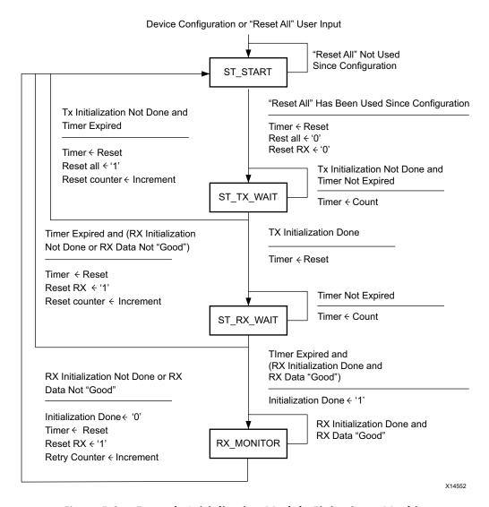
Figure 5-3: Example Initialization Module Finite State Machine
