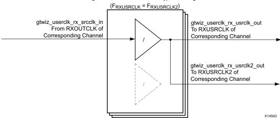
Figure 3-4: Receiver User Clocking Network Helper Block (with One BUFG\_GT)
