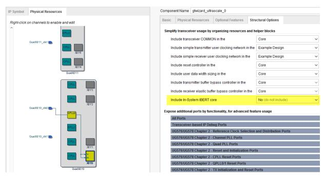
Figure 5-4: Optional enablement of In-System IBERT Core in GT Wizard Example Design
