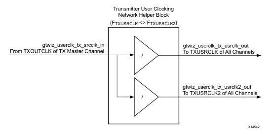
Figure 3-3: Transmitter User Clocking Network Helper Block
