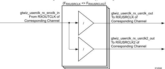
Figure 3-5: Receiver User Clocking Network Helper Block (with Two BUFG\_GT Primitives)
