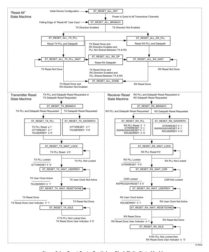
Figure 3-1: Reset Controller Helper Block Finite State Machines
