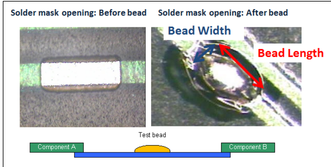
Figure 89. Bead Formed Over Solder-Mask Opening
